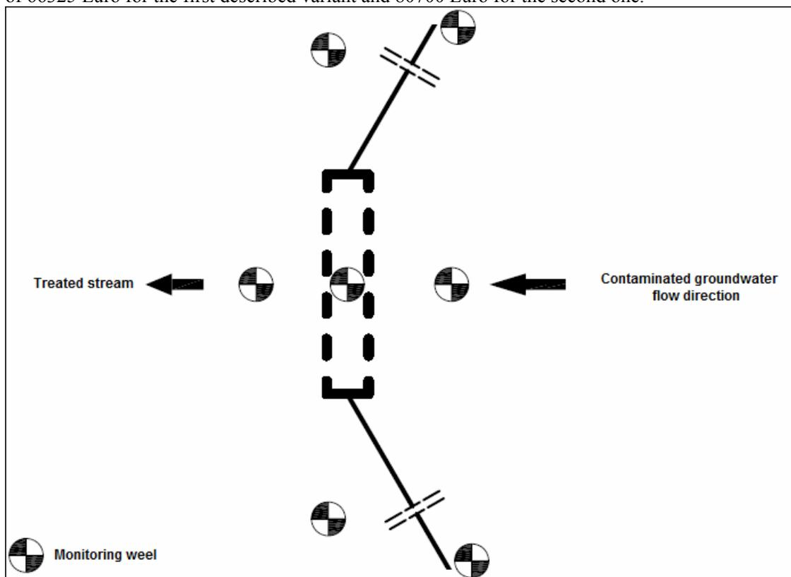
Figure 5: The positioning monitoring wells during the system's operation period scheme.
