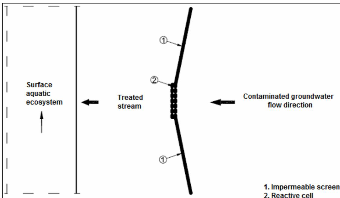
Figure 2: The principle scheme of the method.
