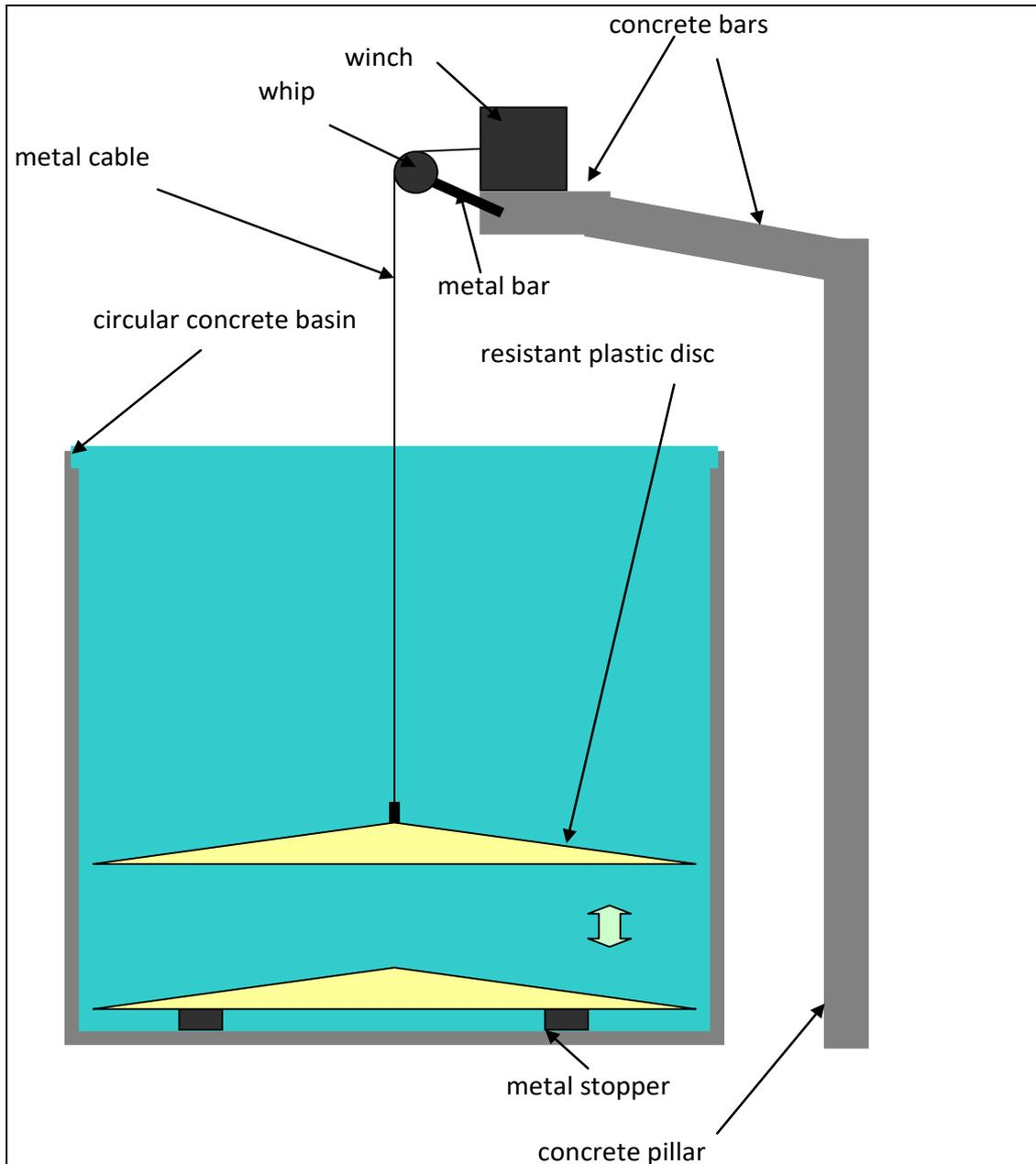
Figure 12: Positioning the winch on the concrete bar (downstream solution) basin - indicative scheme.
