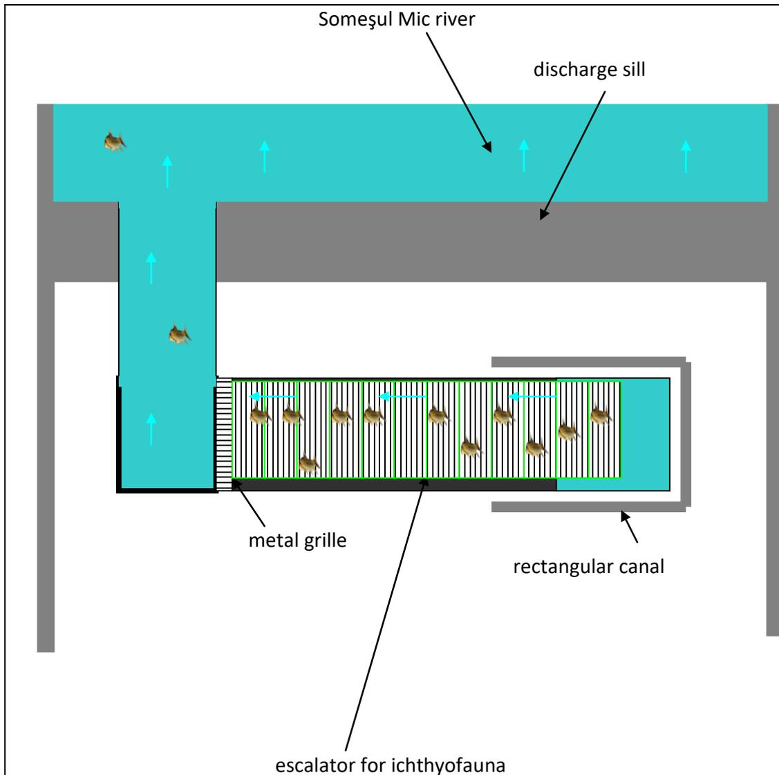
Figure 18: Positioning the escalator (horizontal plane)
