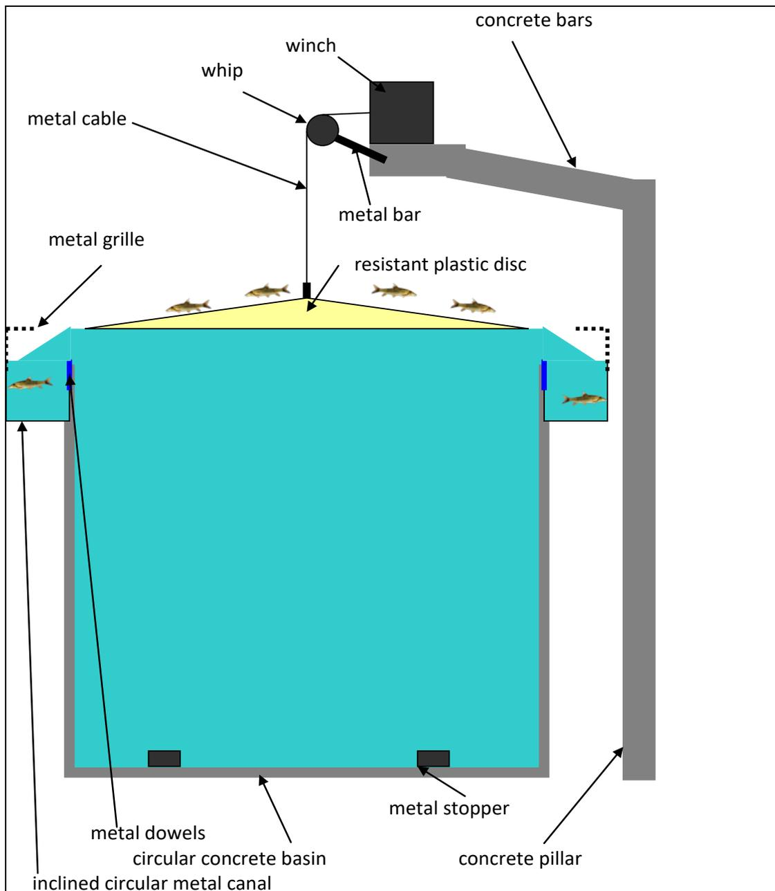
Figure 13: Positioning the circular metal canal basin
