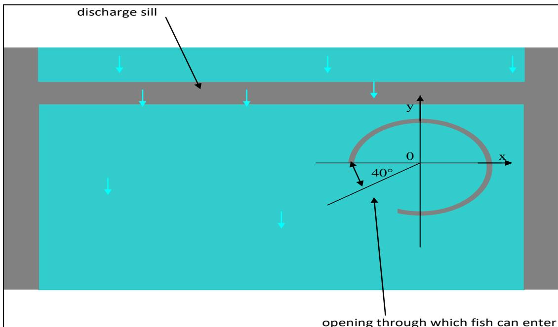
Figure 4: Positioning the circular concrete basin and opening through which fish can enter basin - indicative scheme.
