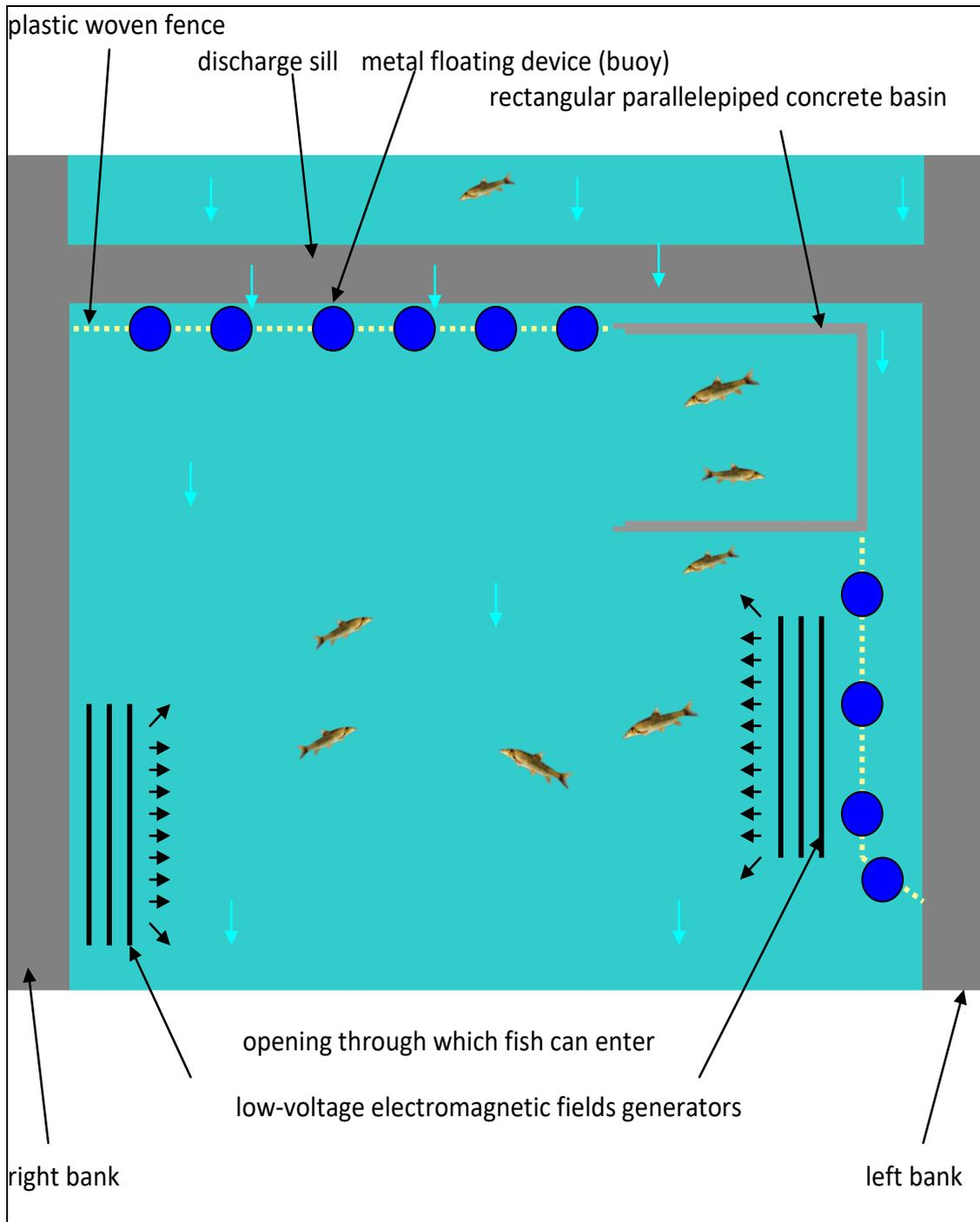
Figure 17: Positioning the rectangular parallelepiped concrete basin.
