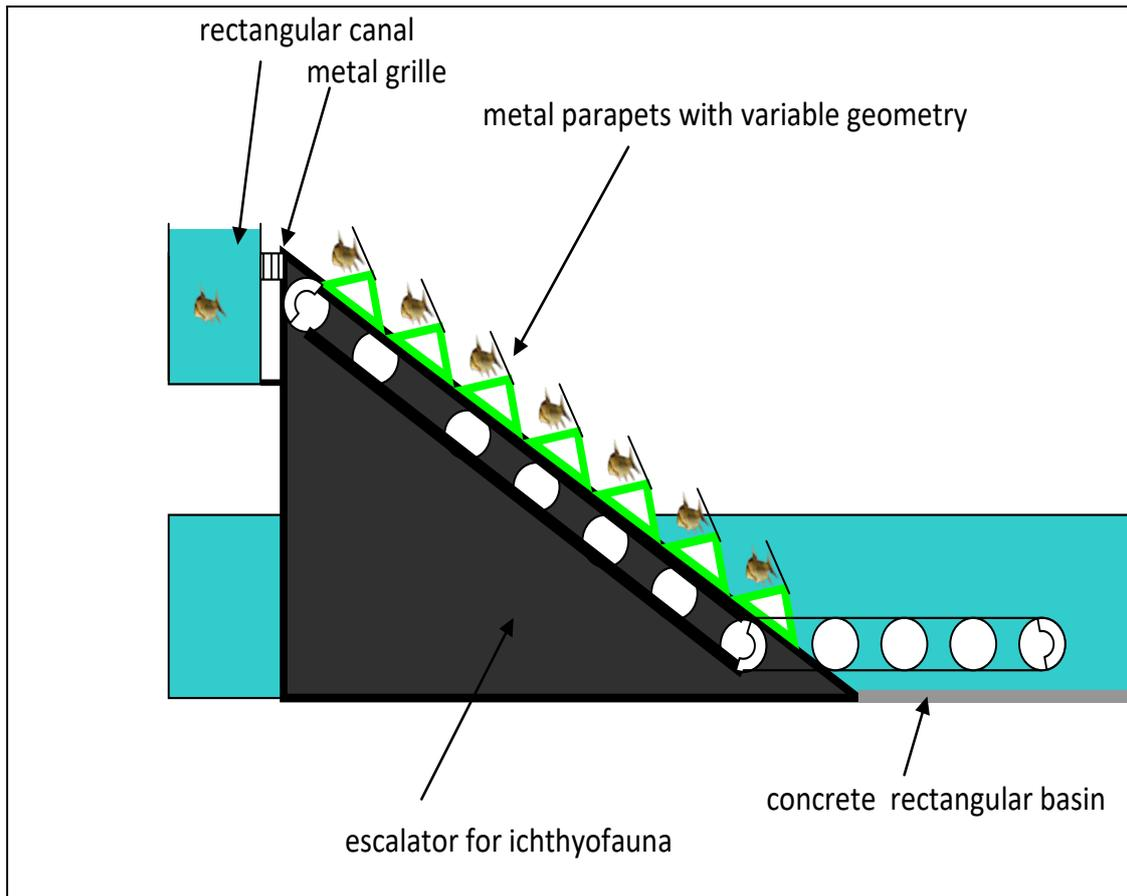
Figure 19: Positioning the escalator (inclined plane)
