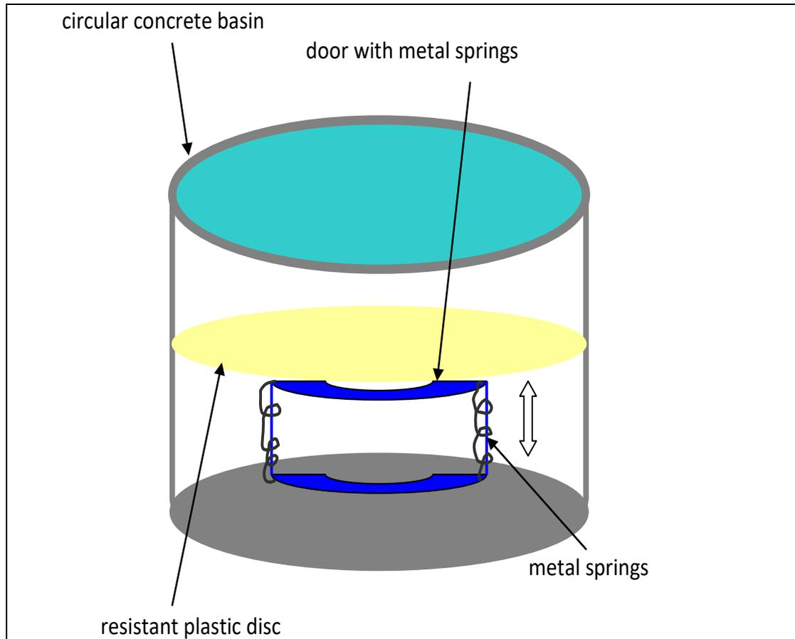
Figure 10: Positioning the fish entrance door of the circular concrete basin
