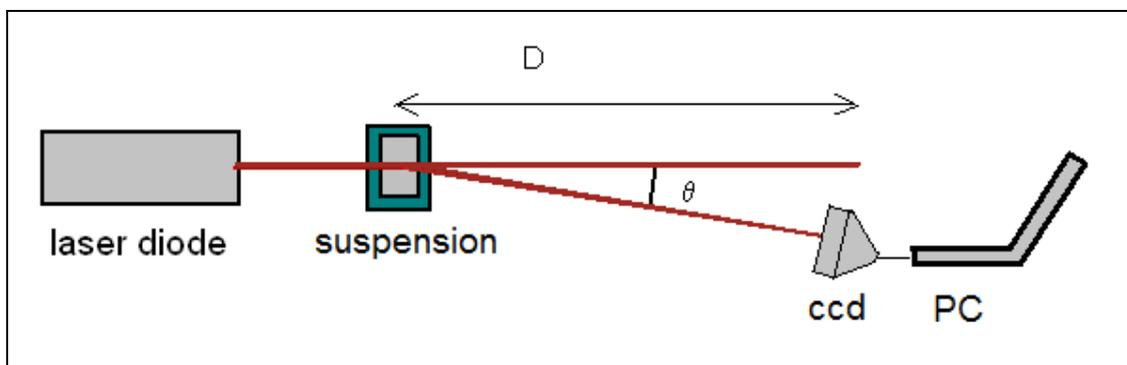
Figure 1: The experiment scheme, above view.
