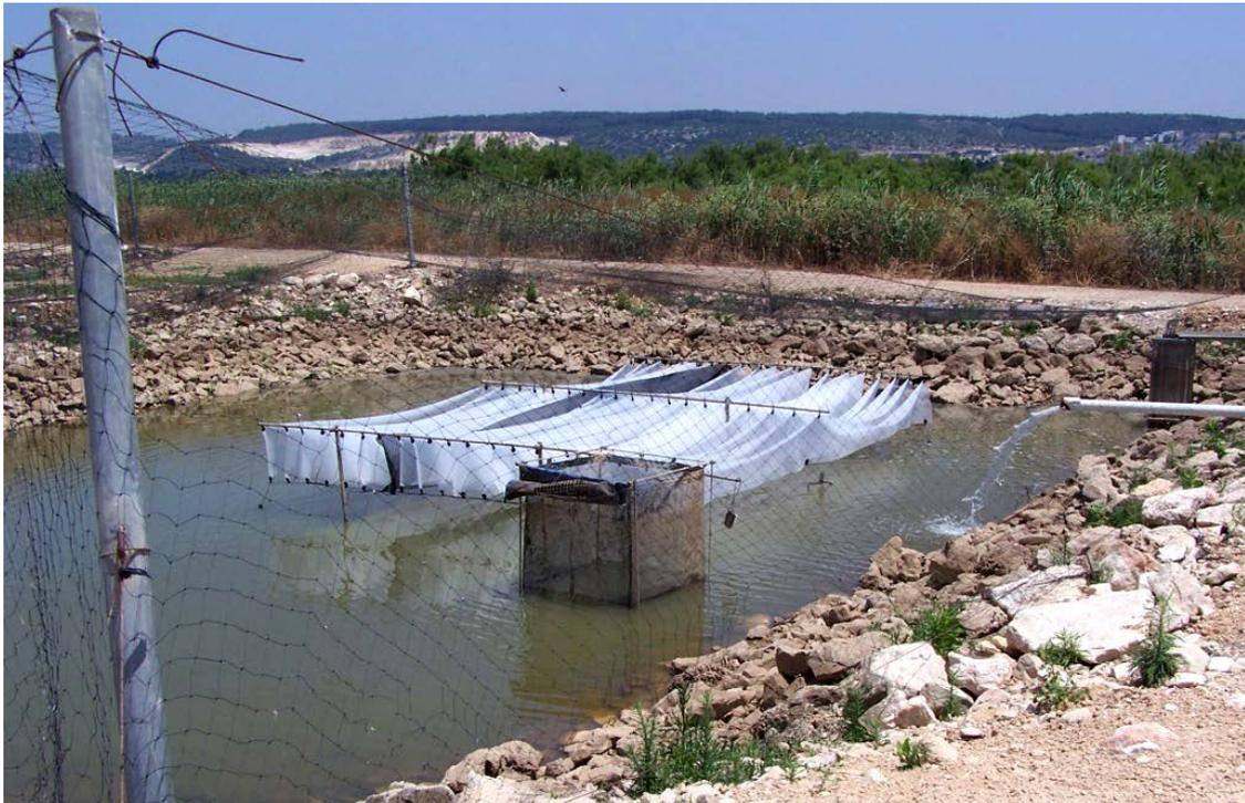
Figure 1: Experimental systems; substrates for periphyton growth in the tilapia culture experiments and the cage in which the substrate experiments were performed; picture taken before the pond was completely filled with water.
