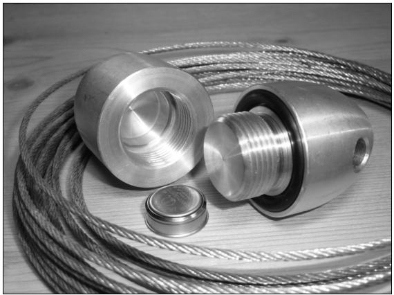
Figure 1: The main components of the Te.M.P.-System, a sensor combined with a battery, a water-tight metal casing and a steel rope to fix the measurement unit.
