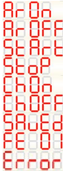
Figure 5. 7 segment display command feedback messages
