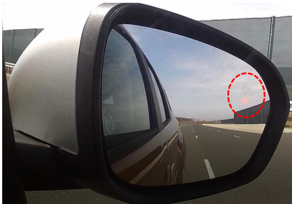
Figure 1. False warning alert example on the tested vehicle [1]
