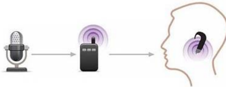
Figure 10. How an FM device system works (MED-EL, 2015)
